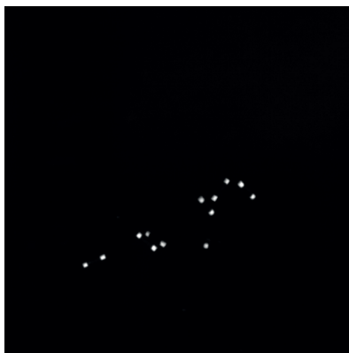
Figure 7.7: Raw image from one of the four cameras in the 3D LPT experiments, the visible white dots represent the ends of the rods. The rods are obtained from the 3D positions of their visible edges using a robust reconstruction algorithm.
